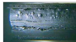
O-ring exposed to rapid depressurization
